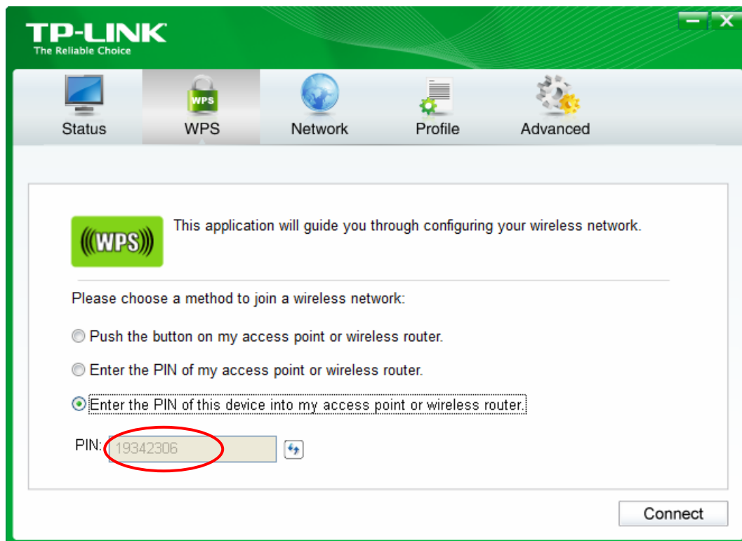
The WPS Configuration Screen of wireless adapter
